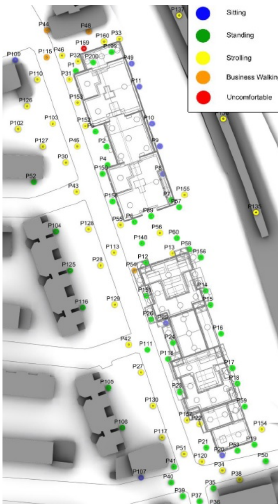
Image 86 (above): Comfort conditions map of the proposed development in the ‘Existing Surrounds, with Mitigation’ scenario
