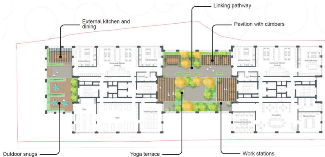
Image 44 (above): Layout of Level 05, showing the two podium-level gardens, which would together provide 460.5 square metres of outdoor amenity space for the PBCL occupiers.
