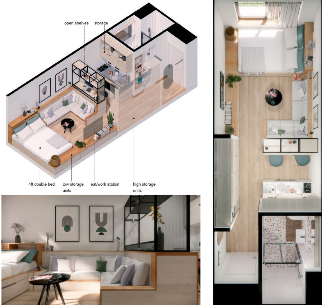
Images 45, 46 and 47 (clockwise from top left): Annotated axonometric, aerial view and visualisation of a Type A1 studio, showing the general layout as well as the typical quality of furnishings and fittings.
